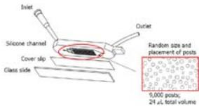
Figure 1. The CEE™ platform utilizes a microfluidic chip to selectively capture and enrich for CTCs. The inclusion of a glass cover slip as part of the CEE™ device allows direct and immediate visual assessment of captured cells, in addition to immunohistochemical and genetic analysis, using standard microscopy. The polymer chip consists of ~9000 posts of variable size/diameter and placement.
